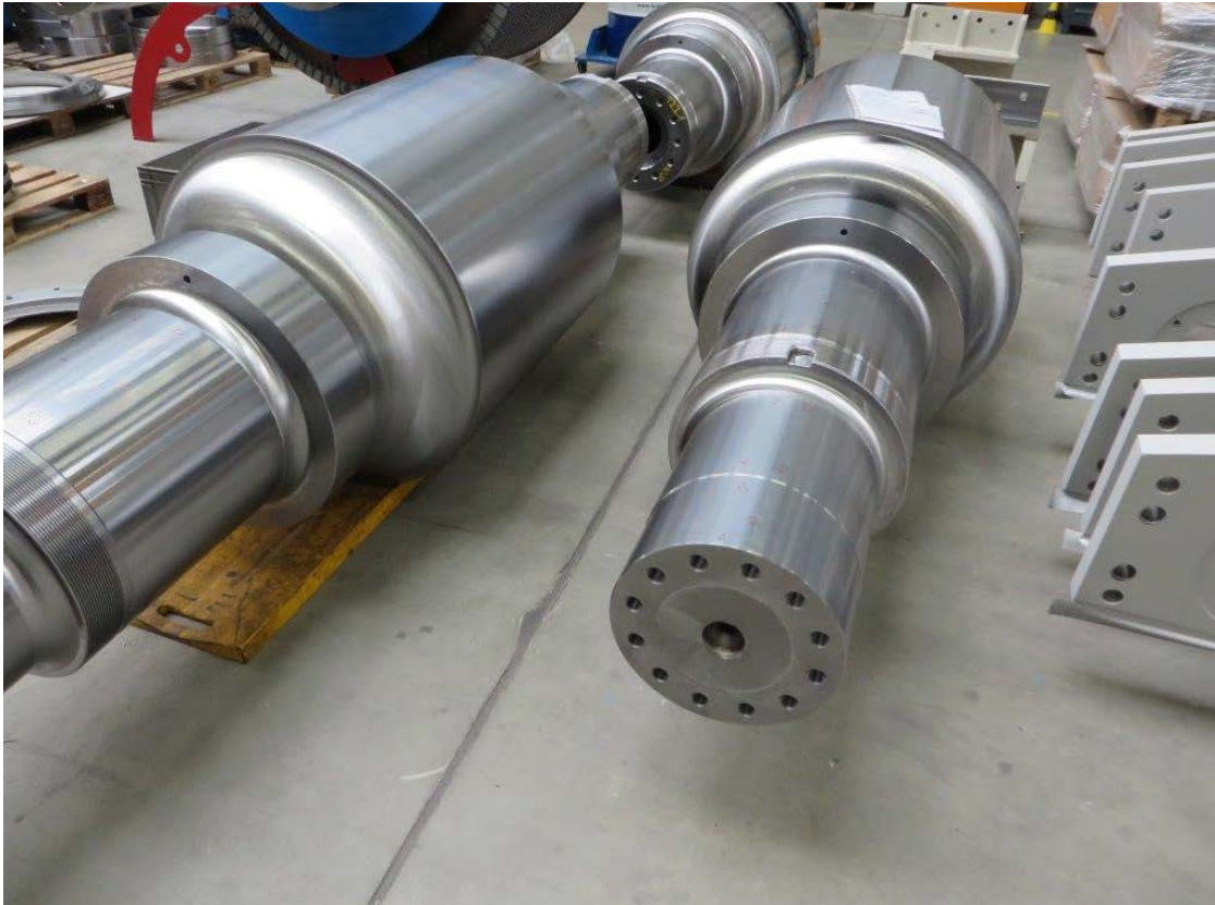
Figure 6: HPGR – Tyre shafts
