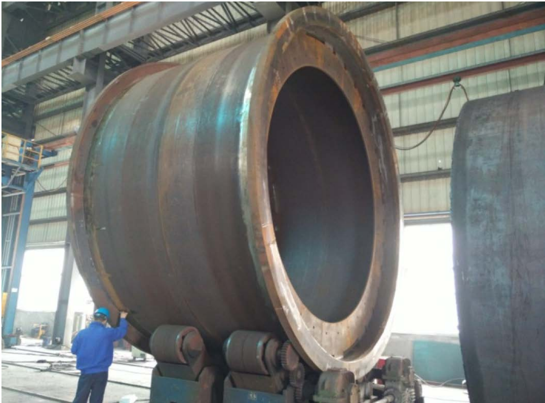
Figure 7: Ball Mill – Mill shell section
