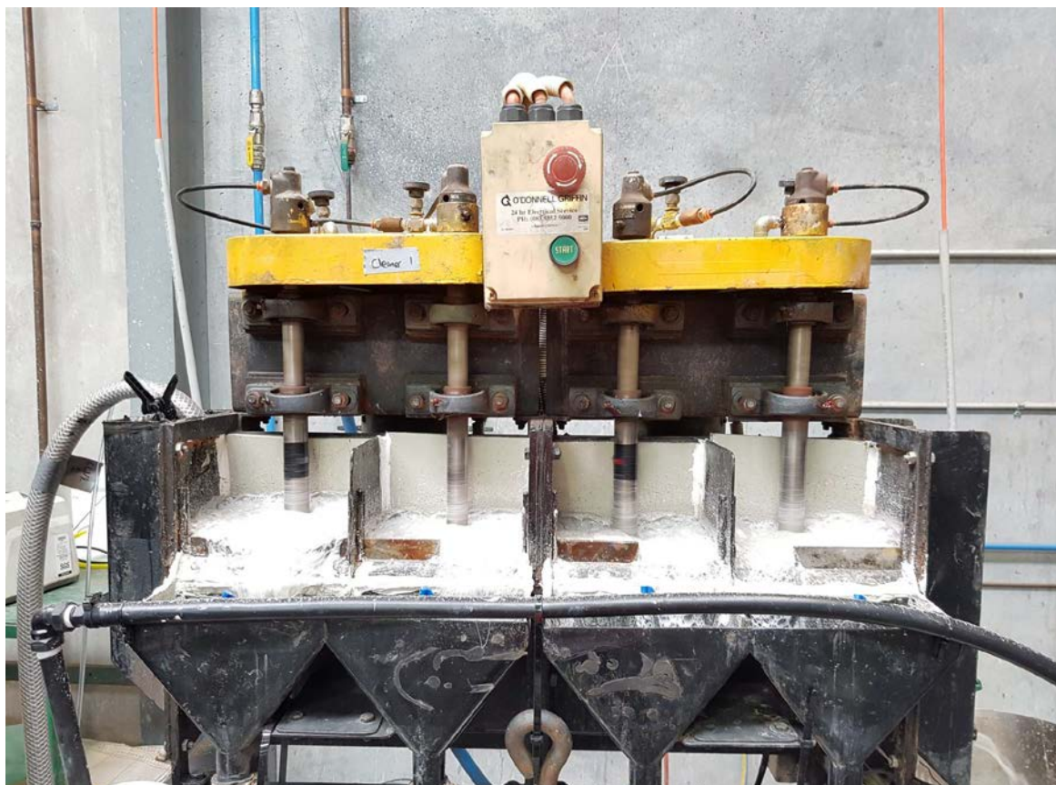
Figure 3: Flotation Pilot Plant – Rougher Cells
